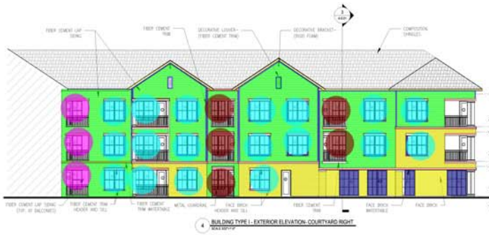
4 BUILDING TYPE I - EXTERIOR ELEVATION COURTYARD RIGHT
